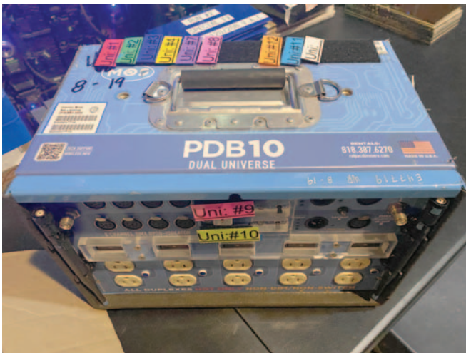
Labels on Velcro tabs allow a stage lighting technician to easily label DMX512 ports to show what universe is being served.
